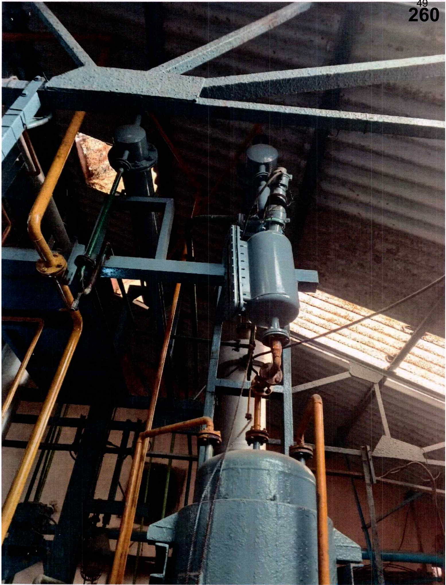
① Double Condensor vent ①
